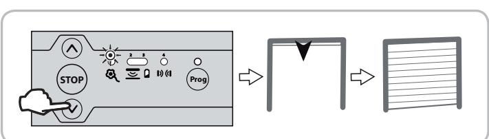
[7]. Press the motor's low end limit push-button.
