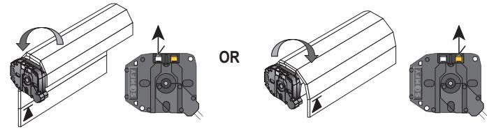
[8]. Press simultaneously on the  $\wedge$  and  $\vee$  buttons or press the  $\text{Prog}$  button until the motor's up and down movement occurs to enter motor adjustment mode.
