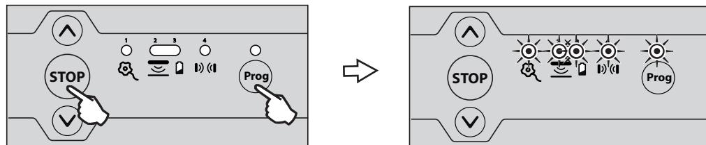
Entry into programming mode by pressing button **Prog** on the receiver is locked.
