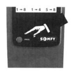
To assign a channel on the receiver (the product is initially configured to operate with the IRT103 transmitter).
