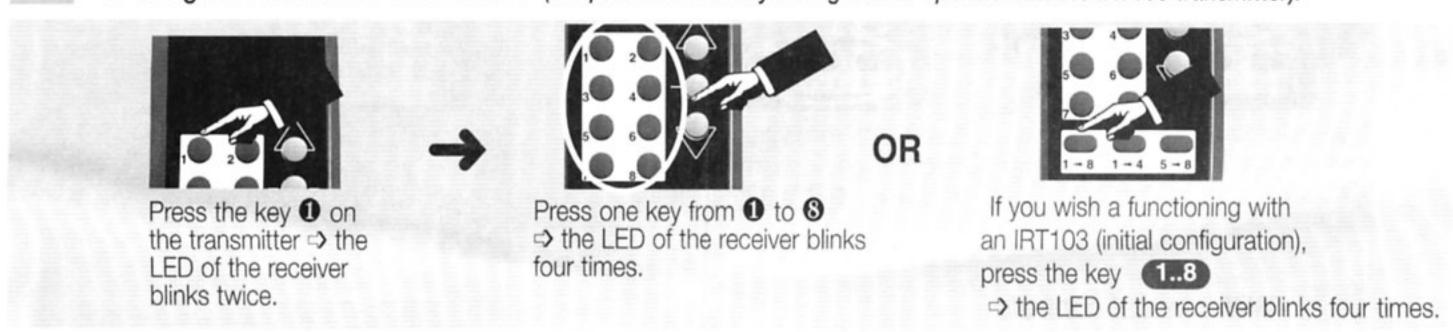
To set the receiver in "Drape" mode (the product is initially configured in "no drape" mode).
