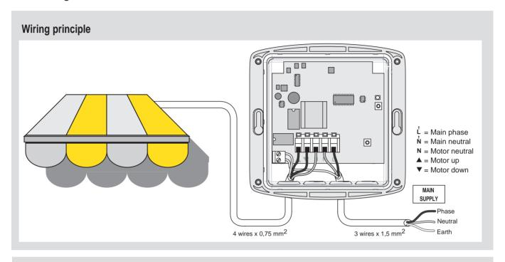
WARNING: if the awning moves DOWN when pressing the UP button of the RTS controls, invert the brown and black motor wires.
