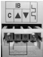
DOWN (C + ▼) The end product should go down
