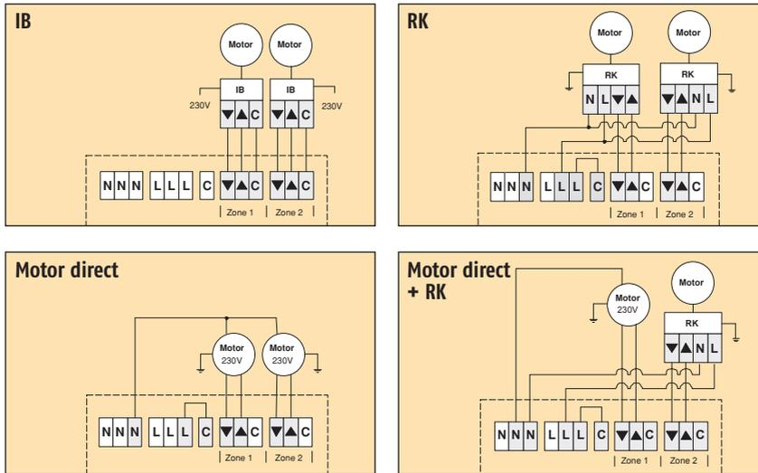
The number of motors that can be connected in RK mode is dependent on the main fuse used. Normally you can count one motor per 1A. This means a 10A fuse allows maximum 10 motors to be connected.
